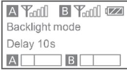
**Set backlight:** Set the background LED light to ON or Delay by 60, 30, or 10 seconds. Default setting is "Delay 30s."
