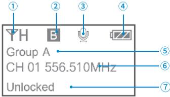
**Home screen.** If no operation is performed for 20 seconds on the other screens, the display will automatically return to the home screen.
