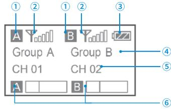
**Home screen:** If no operation is performed for 20 seconds on the other screens, the display will automatically return to the home screen.
