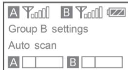
**Auto scan function:** Automatically scan an available and clear channel. For details of operation, please refer to "Using the auto scan function" (page 9).
