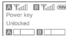
**Power key:** Long press the SET button to unlock or lock the power key. Lock the power key to prevent the receiver being turned off accidentally while in use.
