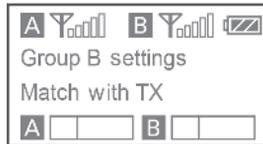
**Infrared matching function:** Match the receiver and transmitter via infrared. For details of operation, please refer to "Matching the receiver and transmitter channel" (page 10).
