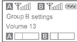
**Set output volume:** Set the volume of output audio within the range of 0 to 15. The setting is retained even after the power is turned off. Default volume is 13.
