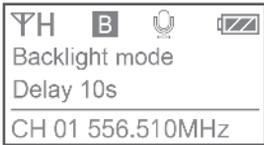
**Set Backlight:** Select ON or Delay by 10, 30, or 60 seconds. The default is "Delay 30s."
