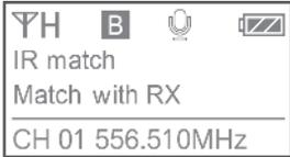
**IR Match:** Set to match with the receiver. The screen will display "Matching" when in process. After successful matching, it will read Match success. If failed to be matched within 20s, the screen displays "Match time out"
