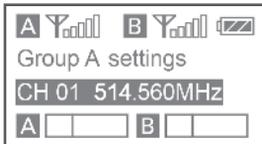
Use the + or - button to select the desired channel and confirm it by short pressing the SET button.
