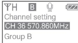
Use the + or - button to select the same channel as the receiver, and confirm it by short pressing the SET button.
