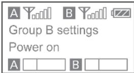
**Channel ON/OFF setting:** You can turn the channel A/B on/off according to your needs.
