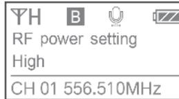
**Select RF power level:** You can set the transmitted RF power to High, Medium or Low. The default is "High."
