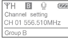
**Select Channel:** Long press the SET button to enter the menu. Use the "+" and "-" to select the channel you need and short press the SET button to confirm.
