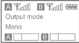
**Output mode:** The output mode can be set to mono or stereo. When the output mode is in mono, the audio from the left and right channel will be mixed. When in stereo, channel A's and channel B's audio output will be separated to the left and right of the stereo output.
